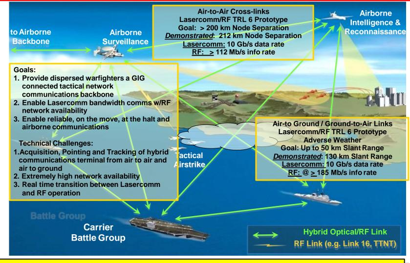
Primary Goal: Demonstrate a four-node hybrid Lasercomm/RF airborne mesh network which provides high availability, high bandwidth, end-to-end connectivity
