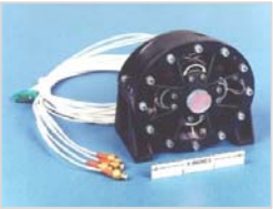
First Space-qualified >1 KHz Tracking Mirror
