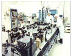
Lasercom Terminal Integration and Full-functional Testing
